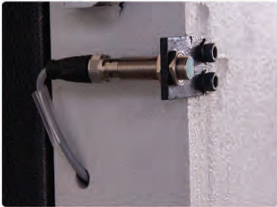
Up-Down Limit Sensors ( Proportional Protect for Sensor Malfunctions)
