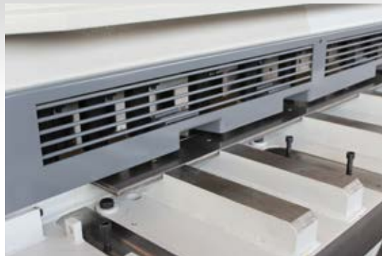
Paramani a greca. Shaped front safety guard.
