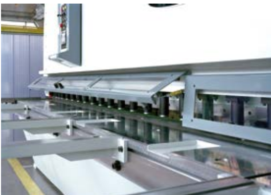
Paramani ribaltabile. Movable swing-up front safety guard.
